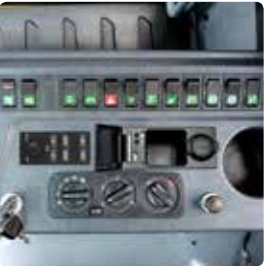
Centralized Instrument Switch Panel
